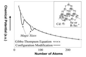
**Fig. 1 Schematic illustration of the relative chemical potential in the small size regime of NPs.** The relative chemical potential of crystals/clusters in the extremely small size regime has dependence of the size and configuration. Adapted with permission from ref. <sup>34</sup>. Copyright 2002 American Chemical Society.
