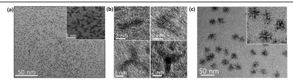
**Fig. 8 Controlling morphology of InP NPs using InP MSCs as precursors.** TEM images of (**a**, **b**) InP BNSs, which were synthesized by the reaction of 386-InP MSCs with In(My)<sub>3</sub> at 220 °C, **c** InP HBNSs/DLNSs which were synthesized by the reaction of 386-InP MSCs with In(Ac)<sub>3</sub> at 220 °C. Adapted with permission from ref. 80. Copyright 2019 The Royal Society of Chemistry.
