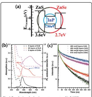
**Fig. 9 Developing the luminescent property of InP MSCs. a** Potential energy diagram for InP, ZnS, and ZnSe bulk materials. **b** UV–vis absorption, PL spectra, and **(c)** PL lifetime of ZnS coated InP MSCs. Adapted with permission from ref. <sup>12</sup>. Copyright 2017 The Royal Society of Chemistry.
